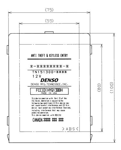
Fig. Marking location and layout of receiver
