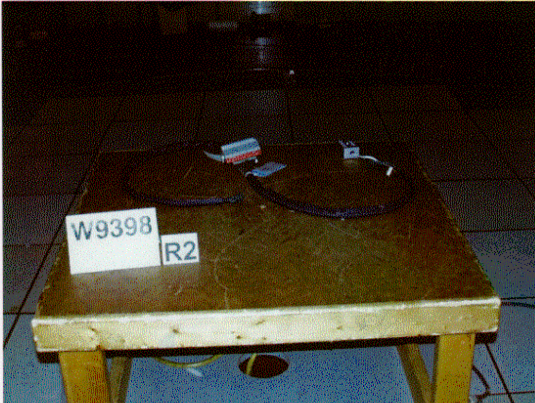
Test-setup photo(s): Radiated emission 30 MHz - 2000 MHz
