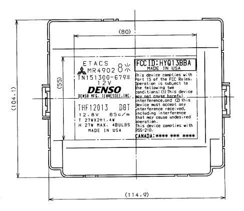
Fig. Marking location and layout of receiver
