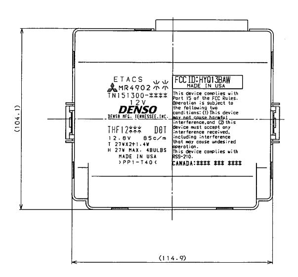
Fig. Marking location and layout of receiver
