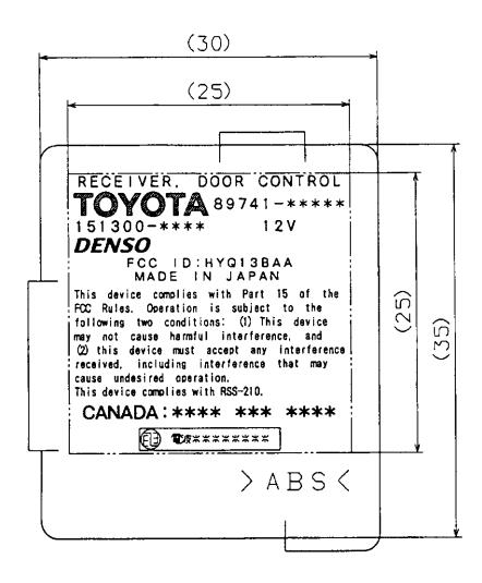
Fig. Marking location and layout of receiver
