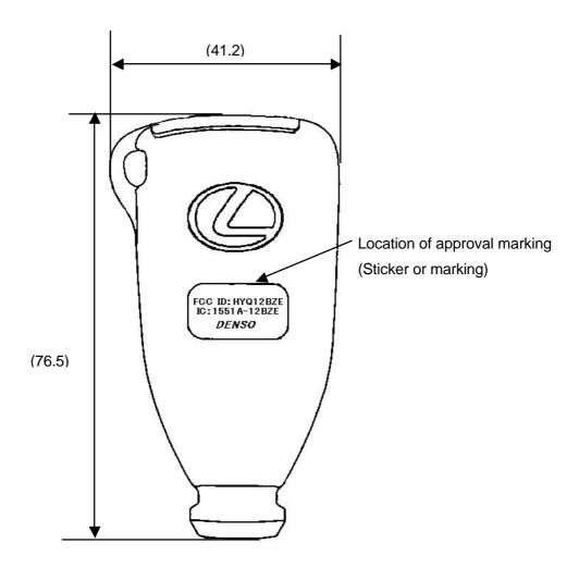
Fig. Marking location and layout of Transmitter
