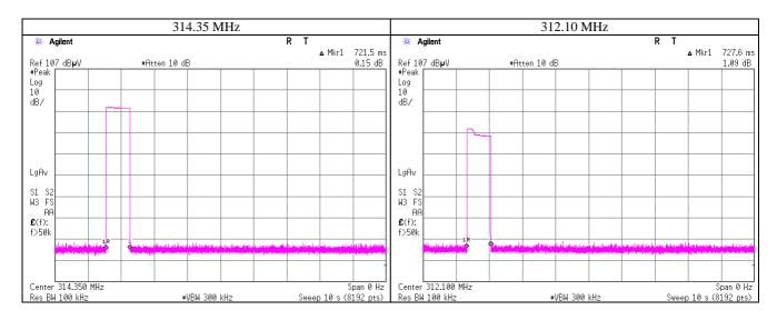
\* The test was performed by a button-pressed operation as representative, because the EUT transmits UHF when LF signal is received from a car or a button on the EUT is pressed, and the UHF transmission is stopped within 5 seconds even when receiving request signal.
