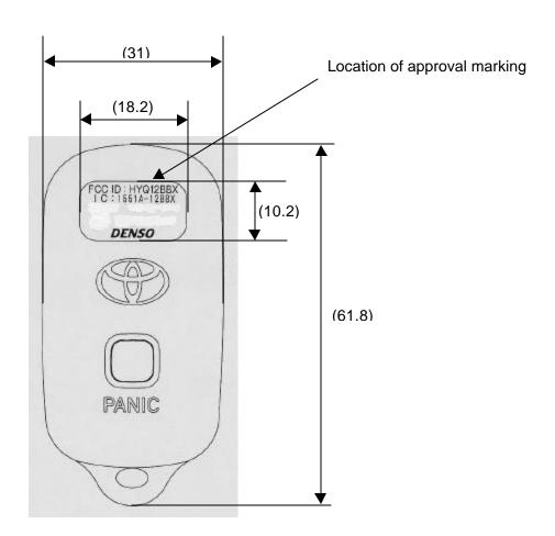
Fig. Marking location and layout of Transmitter
