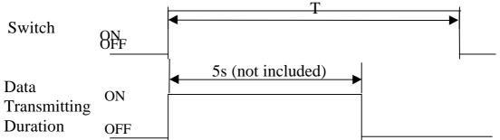
When the switch is pressed for more than 5s, the transmitter stops sending the sdata in 5s (not included) from switch ON. (Auto-power off function)
