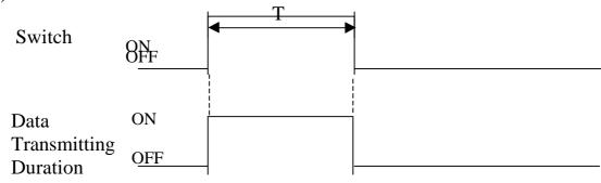
The transmitter sends the data while the switch is pressed.
