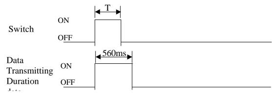
The transmitter sends the data till 560ms from the switch ON.
