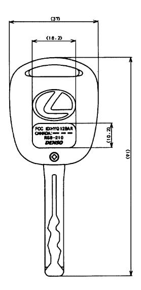
Fig. Marking location and layout of Transmitter
