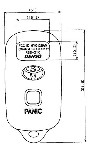
Fig. Marking location and layout of Transmitter
