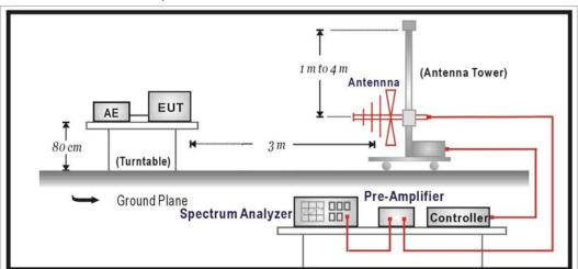
Above 1GHz Test Setup:
