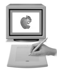
Erasing. In supporting applications, the pen's eraser works like the eraser on a pencil. In text applications, use the eraser to select text, then lift the eraser from the tablet to delete the text.
