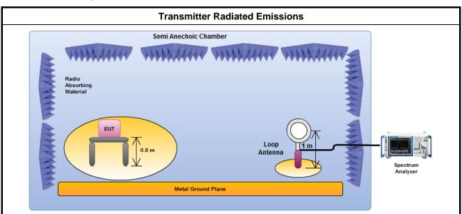
Magnetic field tests shall be performed in the frequency range of 9 kHz to 30 MHz using a calibrated loop antenna. The center of the loop shall be 1 m above the ground.
