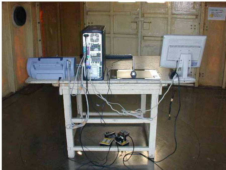
Setup with the Maximized RFI Field Strength Emission Level (PTZ-930 + Airbrush)
