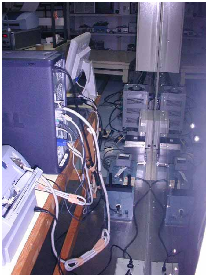
Setup with the Maximized RFI Voltage Emission Level (PTZ-930 + 2D Mouse)
