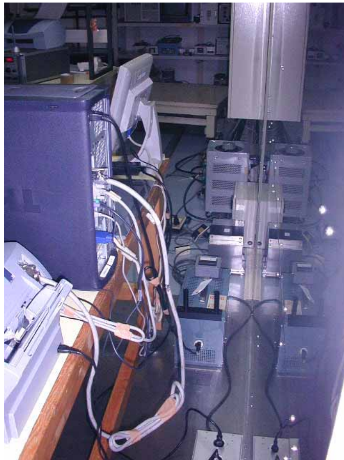
Setup with the Maximized RFI Voltage Emission Level (PTZ-930 + Airbrush)
