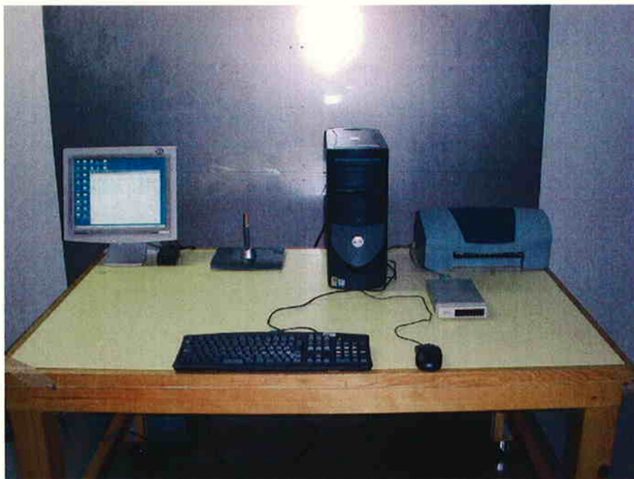
Photo 7.1a Setup with the Maximized RFI Voltage Emission Level (PTZ-430 + Grip Pen)
