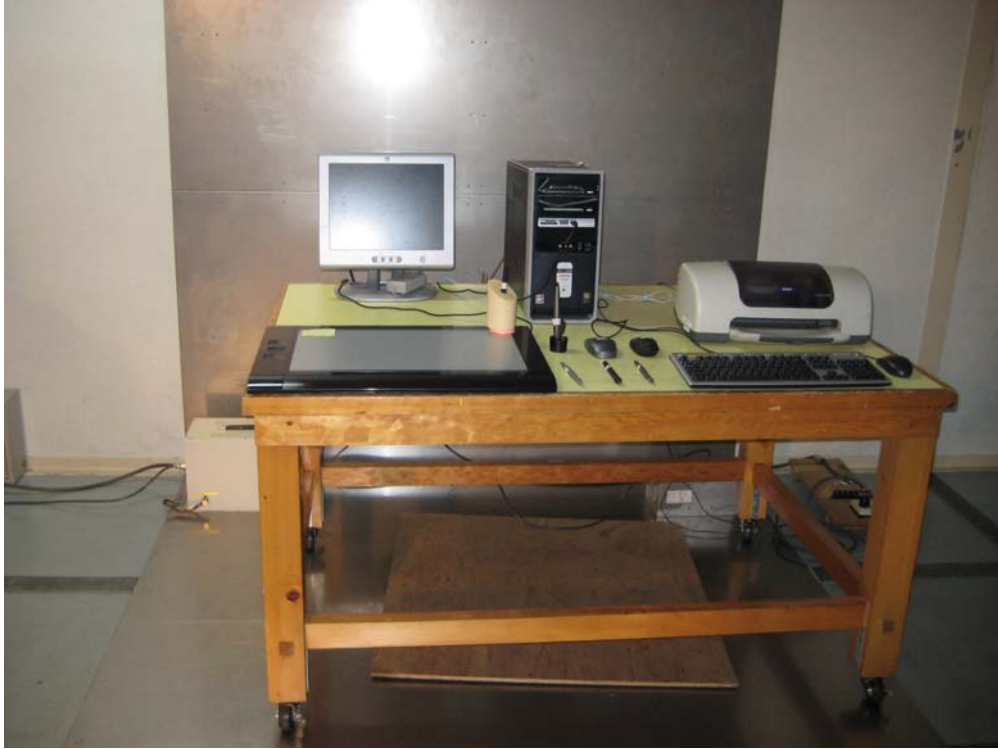
Photo 7.1 Setup with the Maximized RFI Voltage Emission Level
