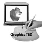
**Erasing.** In supporting applications, the pen's eraser works like the eraser on a pencil. In text applications, use the eraser to select text, then lift the eraser from the tablet to delete the text
