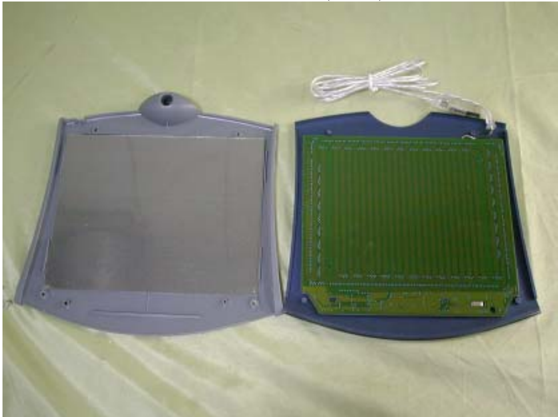
Internal Photo of EUT ( Tablet )
