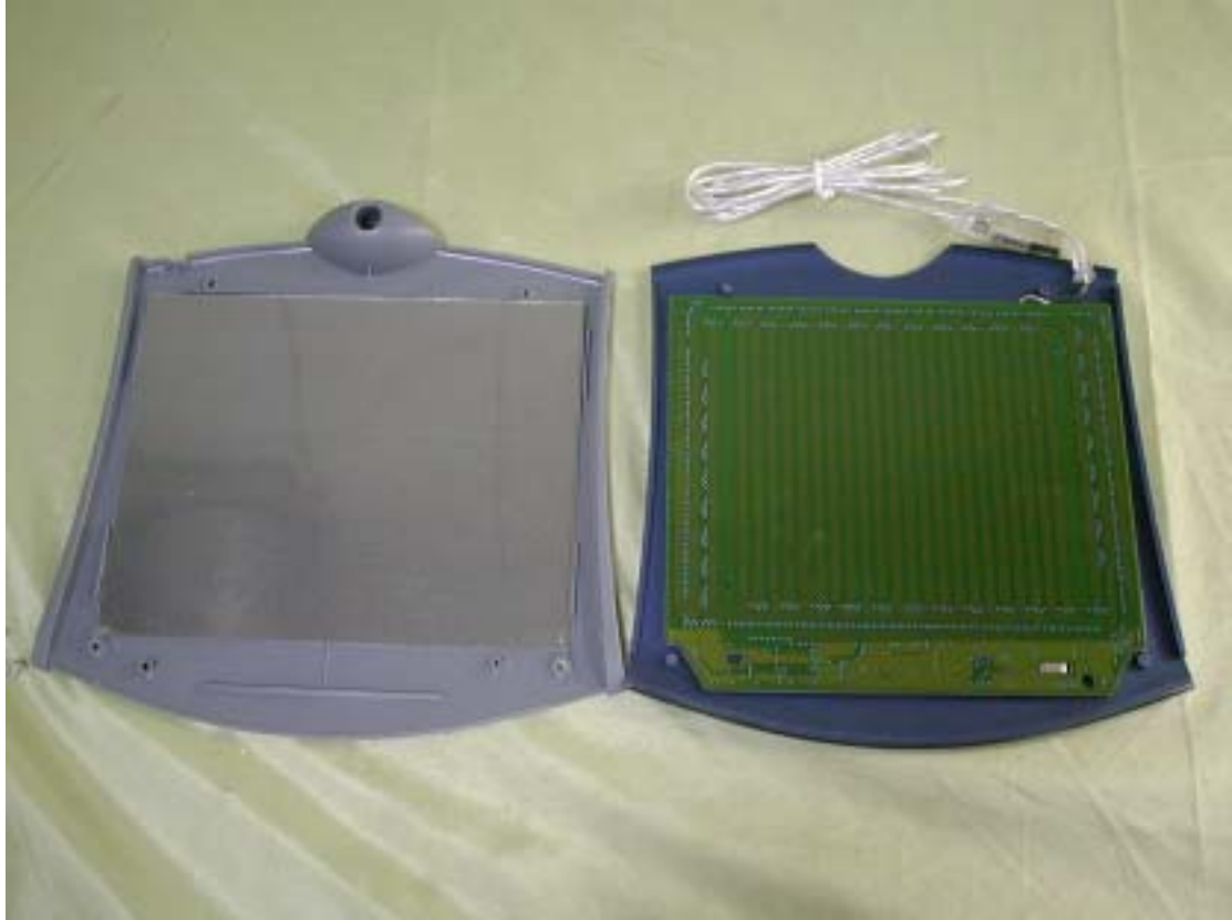
Internal Photo of EUT ( Tablet )
