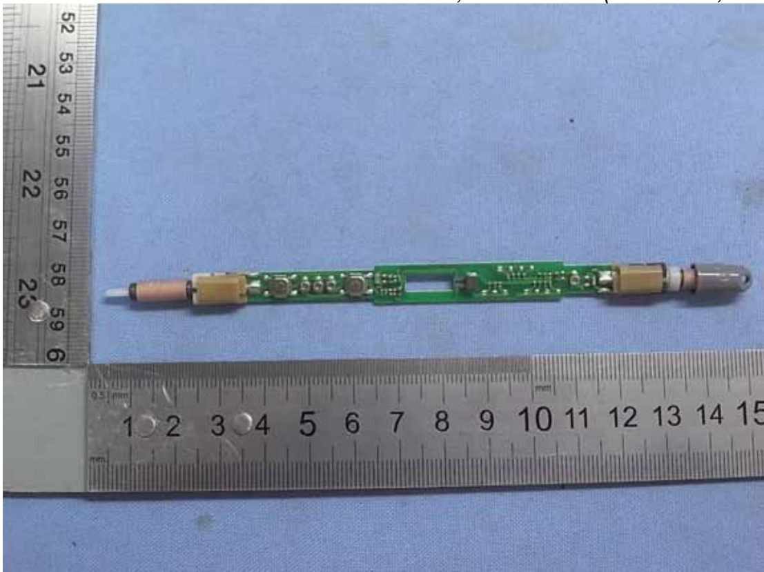
Figure 39 Pen, Internal View (TX Module, Front View)
