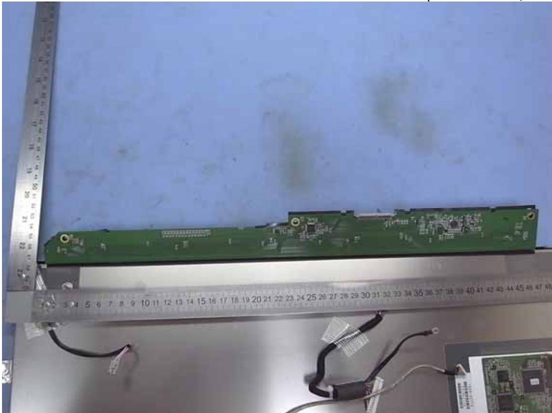
Figure 37 Internal View (LVDS Board, Back View)
