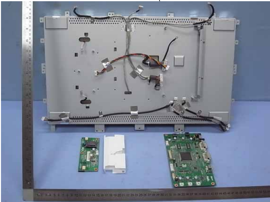
Figure 25 Internal View (Removed Main Board & Inverter Board)
