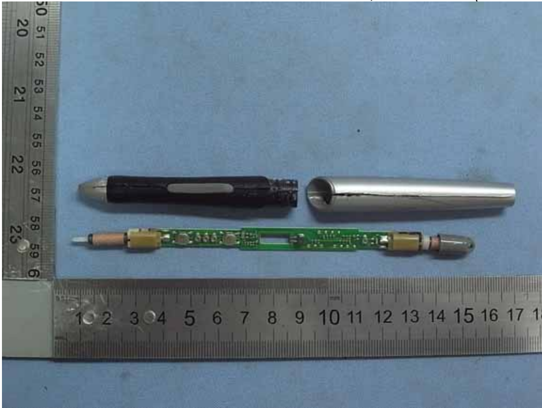
Figure 39 Pen, Internal View (TX Module, Front View)
