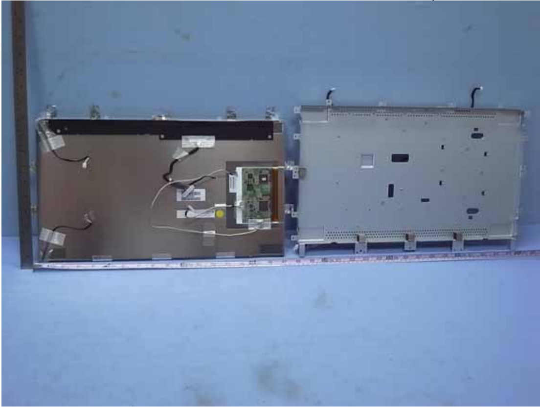
Figure 33 Internal View (LCD Panel, Back View)
