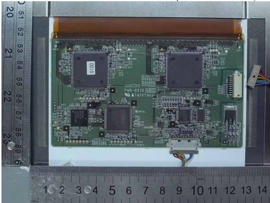
Figure 35 Internal View (Sensor Control Board, Back View)
