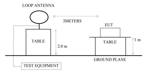
3.2.3. Semi-Anechoic Chamber (3m) Setup Diagram for 30-1000MHz
