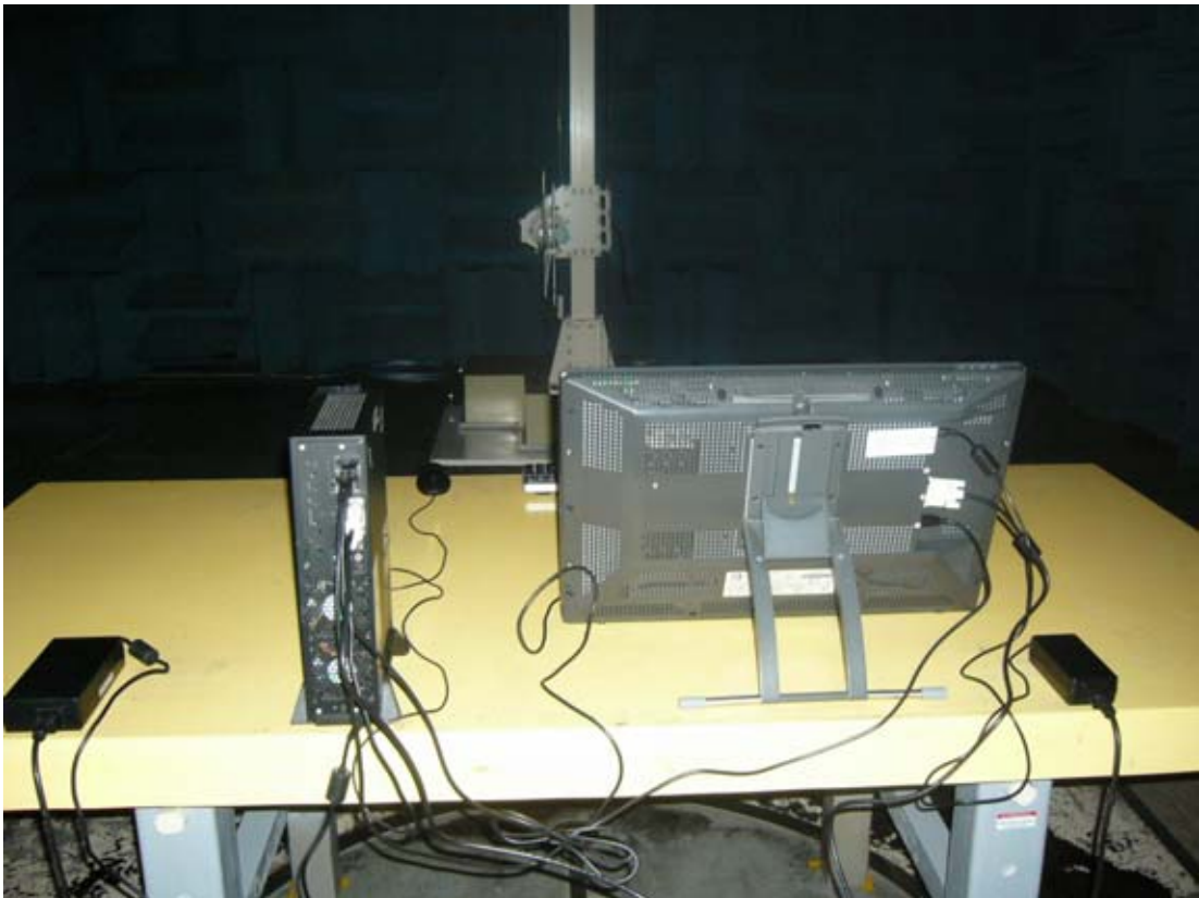
BACK VIEW OF RADIATED MEASUREMENT
