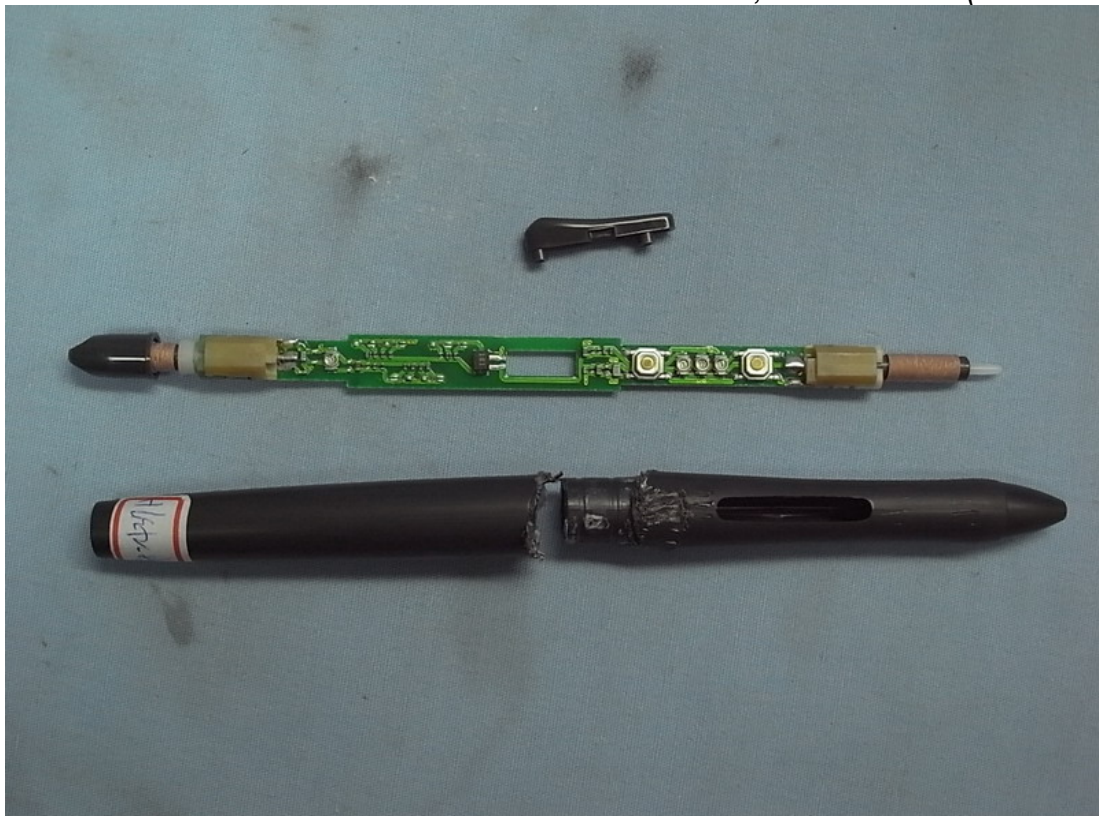
Figure 29 Pen, Internal View (Removed Cover)
