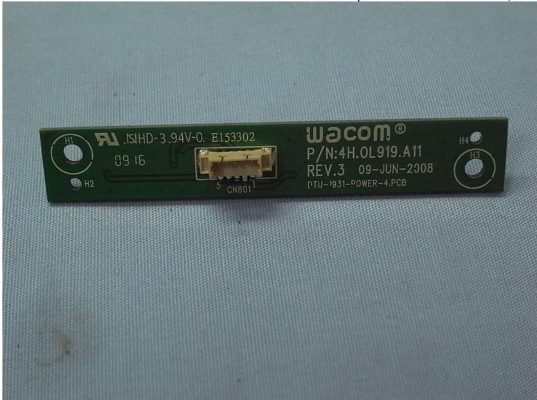
Figure 12 Internal View (Switch Control Board, Back View)
