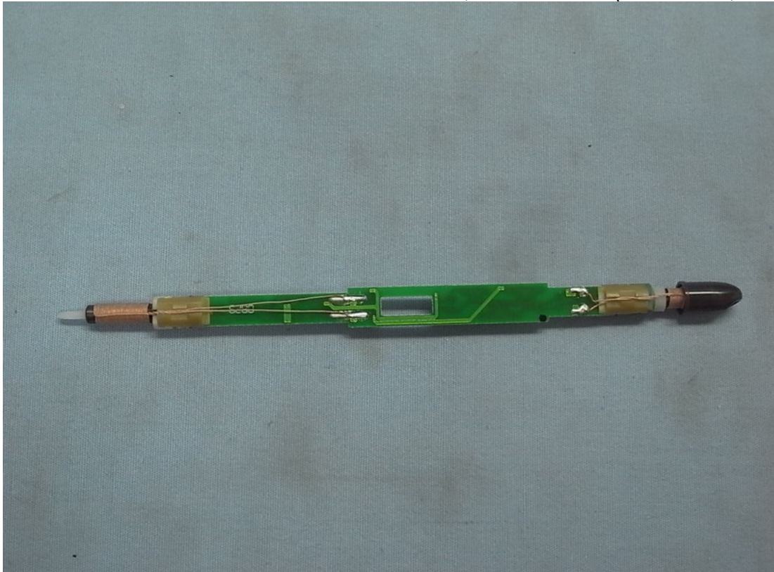
Figure 31 Pen, Internal View (TX Module, Back View)
