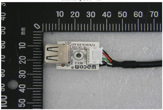
Internal of EUT – 17 (Antenna)
