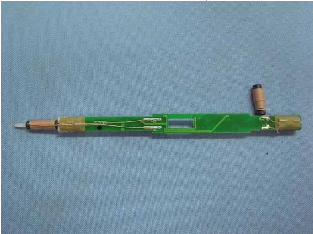
Figure 33 Pen, Internal View (TX Module, Back View)
