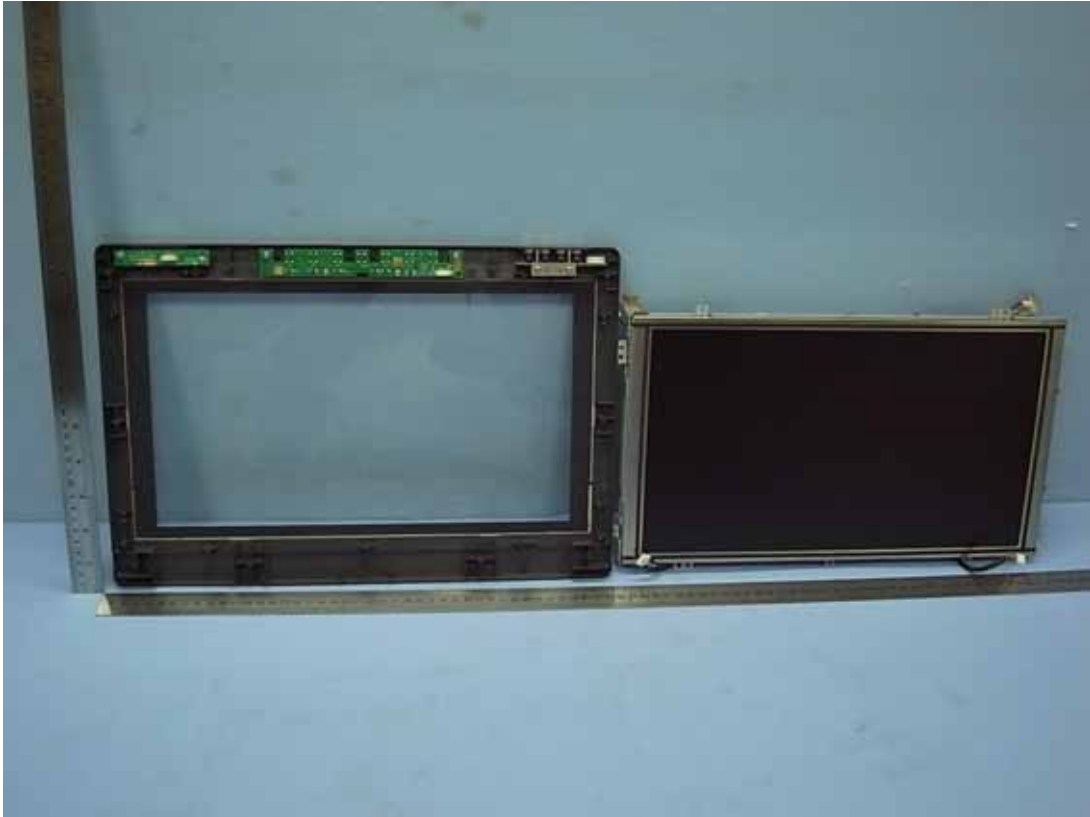
Figure 11 Internal View (Removed Front Frame, LCD Panel, Front View)
