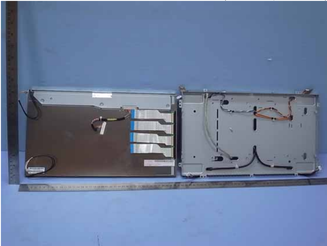
Figure 31 Internal View (LCD Panel, Back View)
