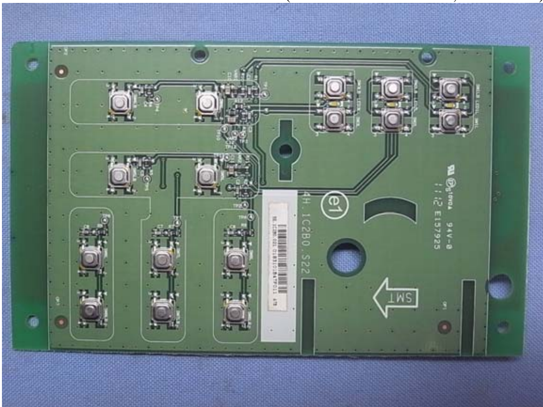
Figure 40 Internal View (Function Control Board, Front View)
