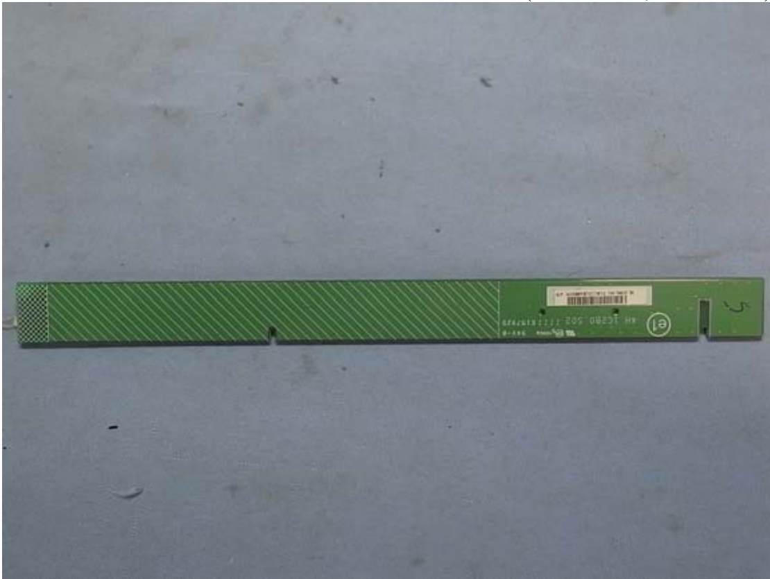
Figure 47 Internal View (OSD Board, Back View)
