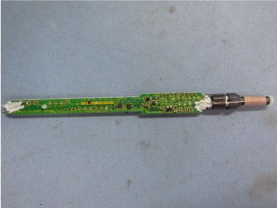
Figure 55 Pen, Internal View (Main Board, Back View)
