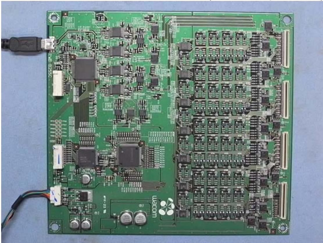
Figure 31 Internal View (Control Board, Front View)
