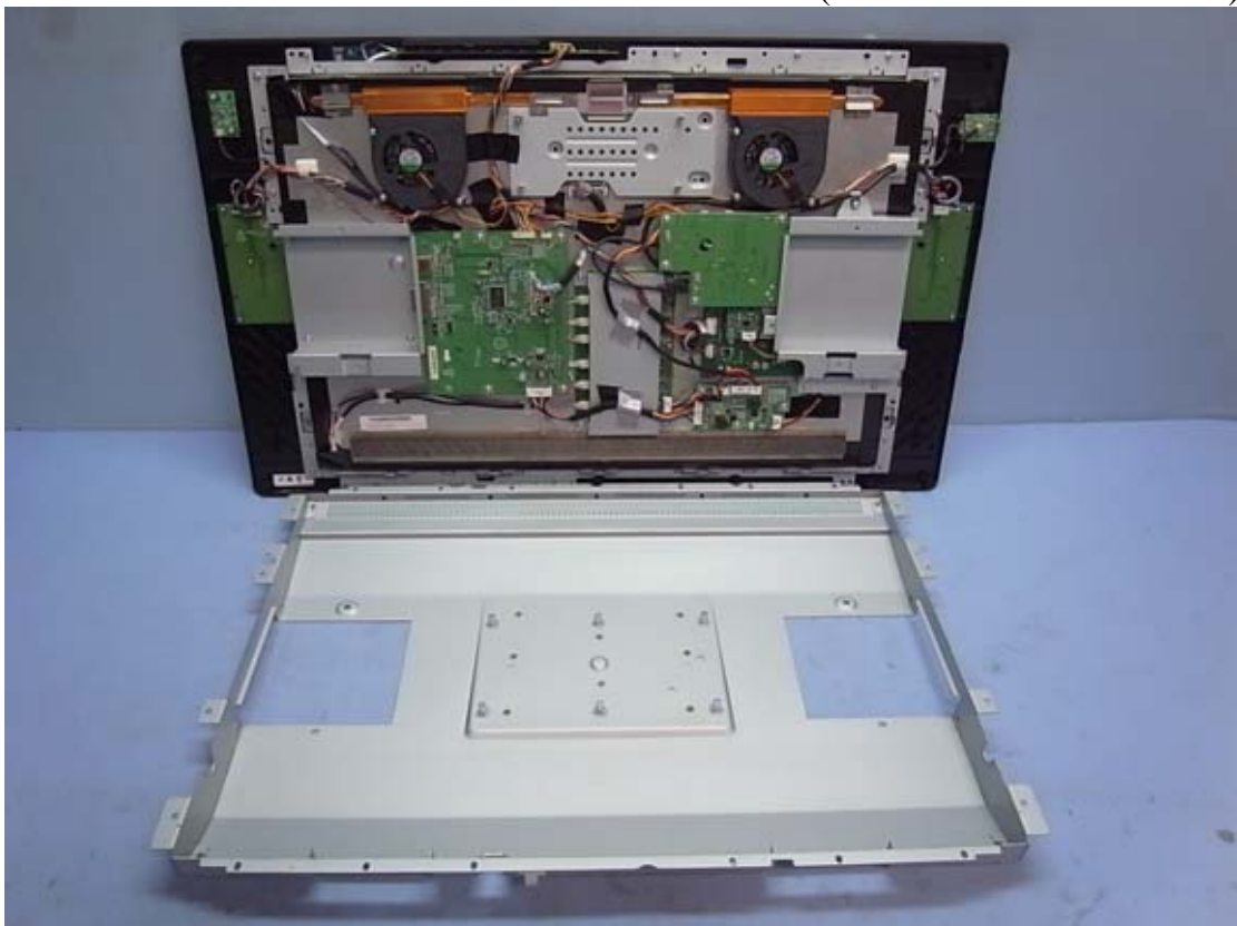
Figure 20 Internal View (Removed Shielded Cover)
