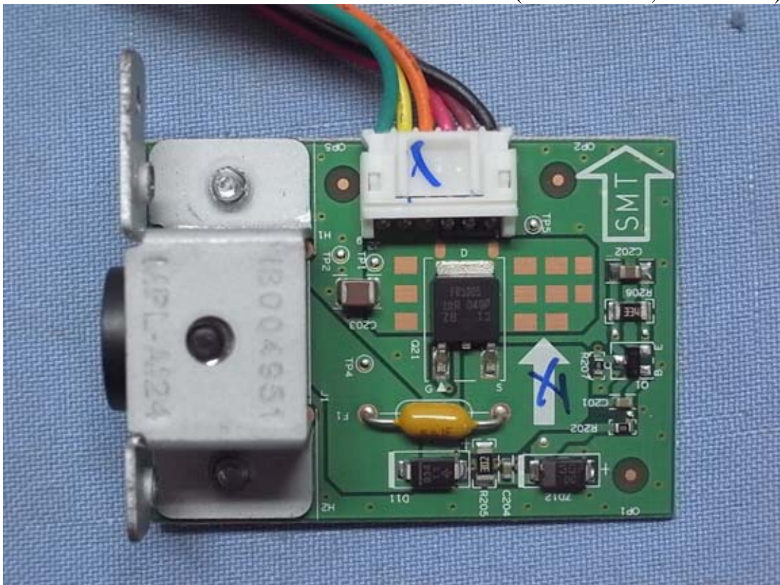
Figure 28 Internal View (Power Board, Front View)
