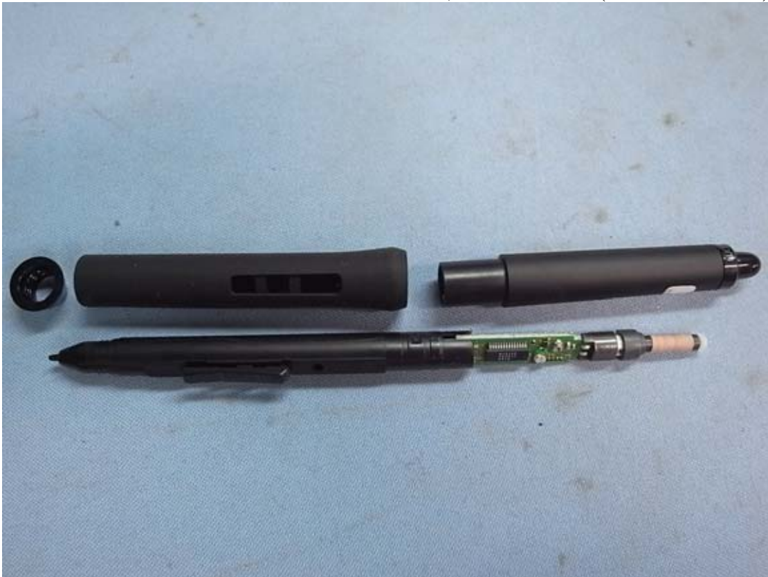
Figure 53 Pen, Internal View (Removed Cover)
