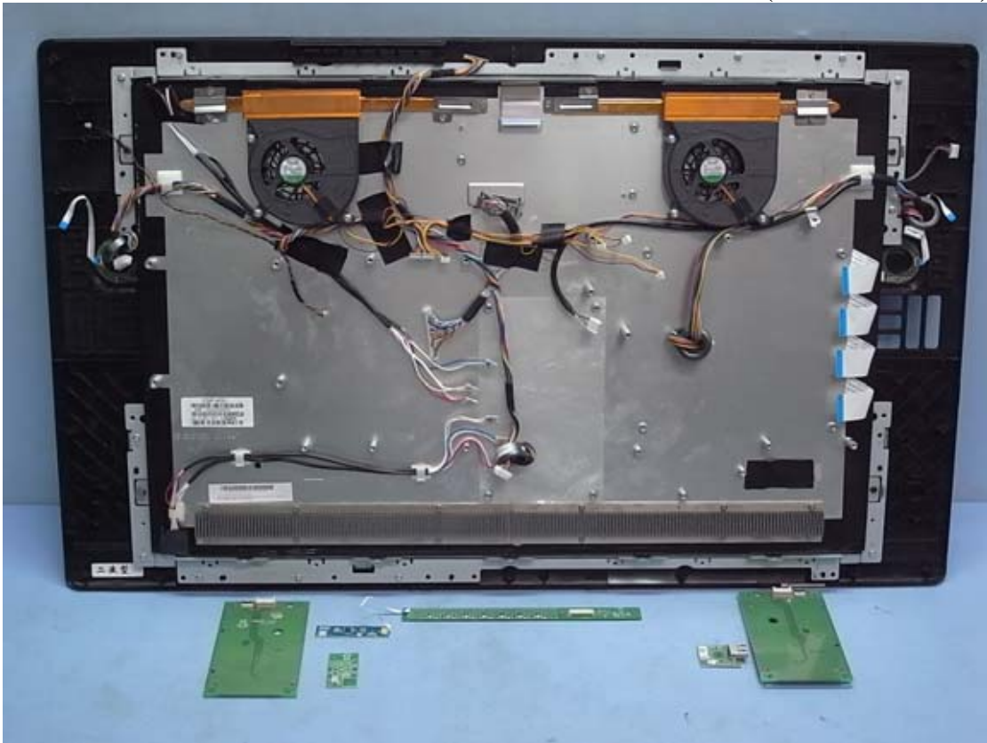
Figure 37 Internal View (Removed PCB's)
