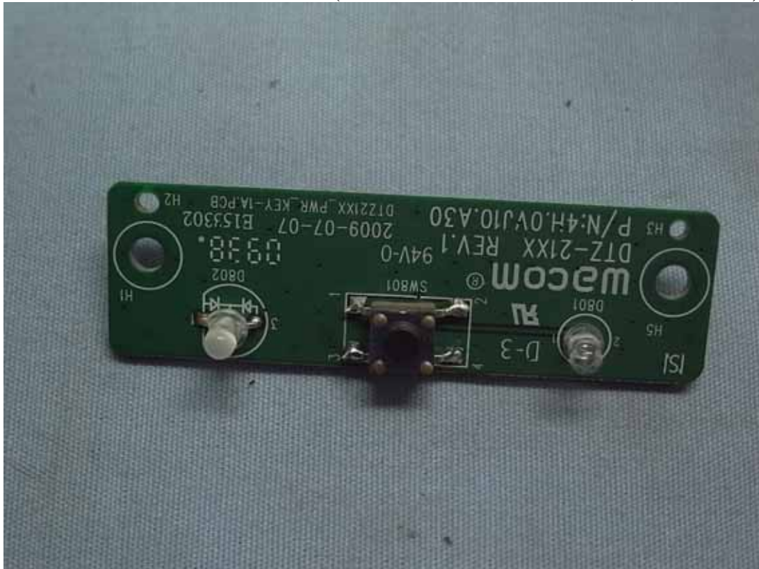
Figure 18 Internal View (Switch Control & LED Board, Front View)
