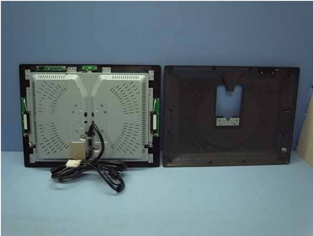
Figure 10 Internal View (Removed Back Cover)
