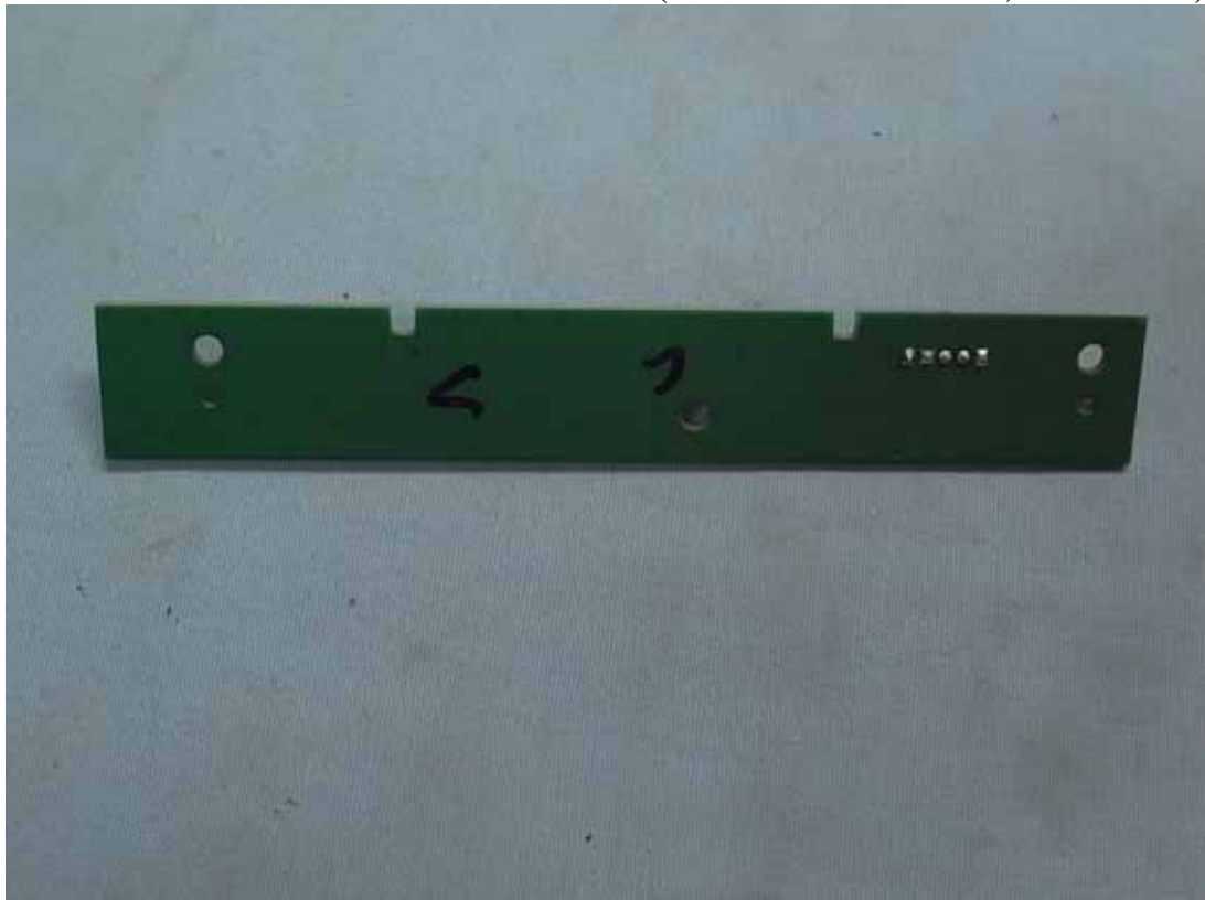
Figure 17 Internal View (Switch Control Board, Back View)
