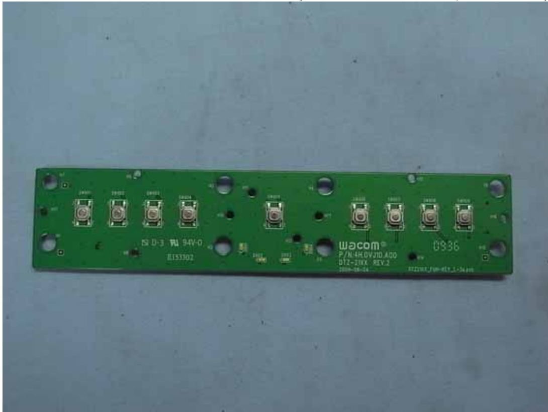
Figure 14 Internal View (Switch Control Board, Front View)
