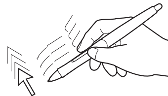
Parallax effect caused by screen glass. Note how the position of the pen tip and screen cursor are not aligned.
