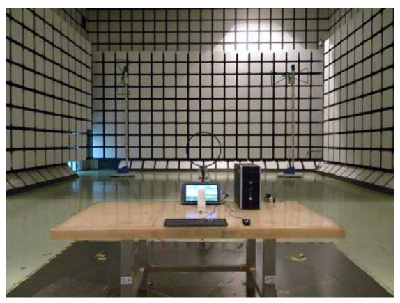
7.3. Photos of radiated emissions 30MHz-1000MHz
