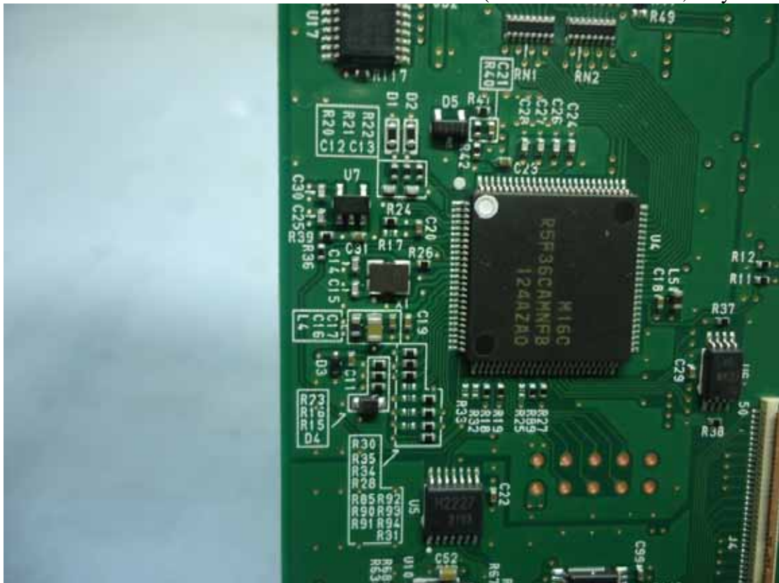
Figure 23 I/O Board#1 (Wacom/ PWB-B779, Crystal oscillator)
