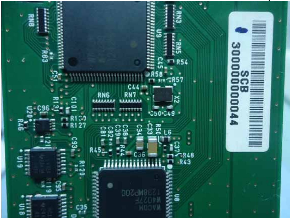
Figure 22 I/O Board#1 (Wacom/ PWB-B779, Crystal oscillator)
