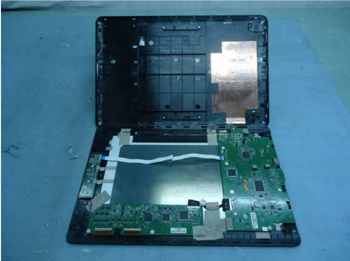
Figure 6 Cover Remove & EMI solution
