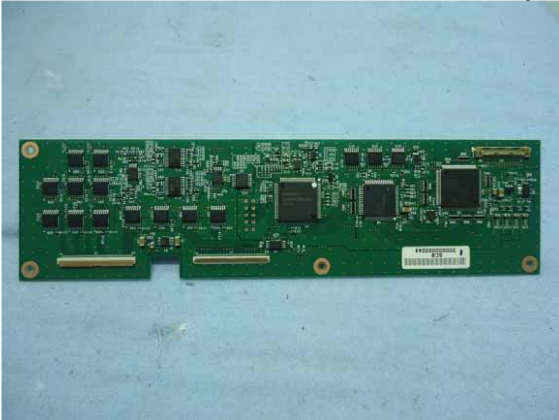
Figure 20 I/O Board#1 (Wacom/ PWB-B779, Component Side)
