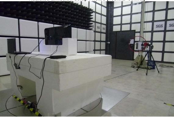
Radiated Emission Setup Photos (30MHz~1GHz)
