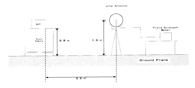
MEASUREMENT SET-UP FOR RADIATED EMISSIONS 30 MHz - 1000 MHz
