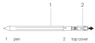
**2.** Insert the battery in the battery holder then attach to the top cover with the positive side of the battery facing the top cover.
