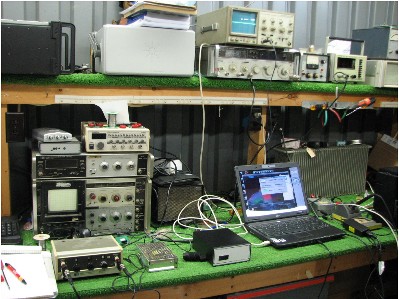
Engineering Laboratory, Test Setup for MTS10W Transmitter Testing
