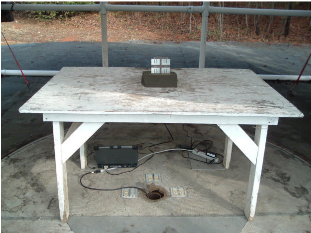
Photograph of Spurious Emissions Patch (Front View)
