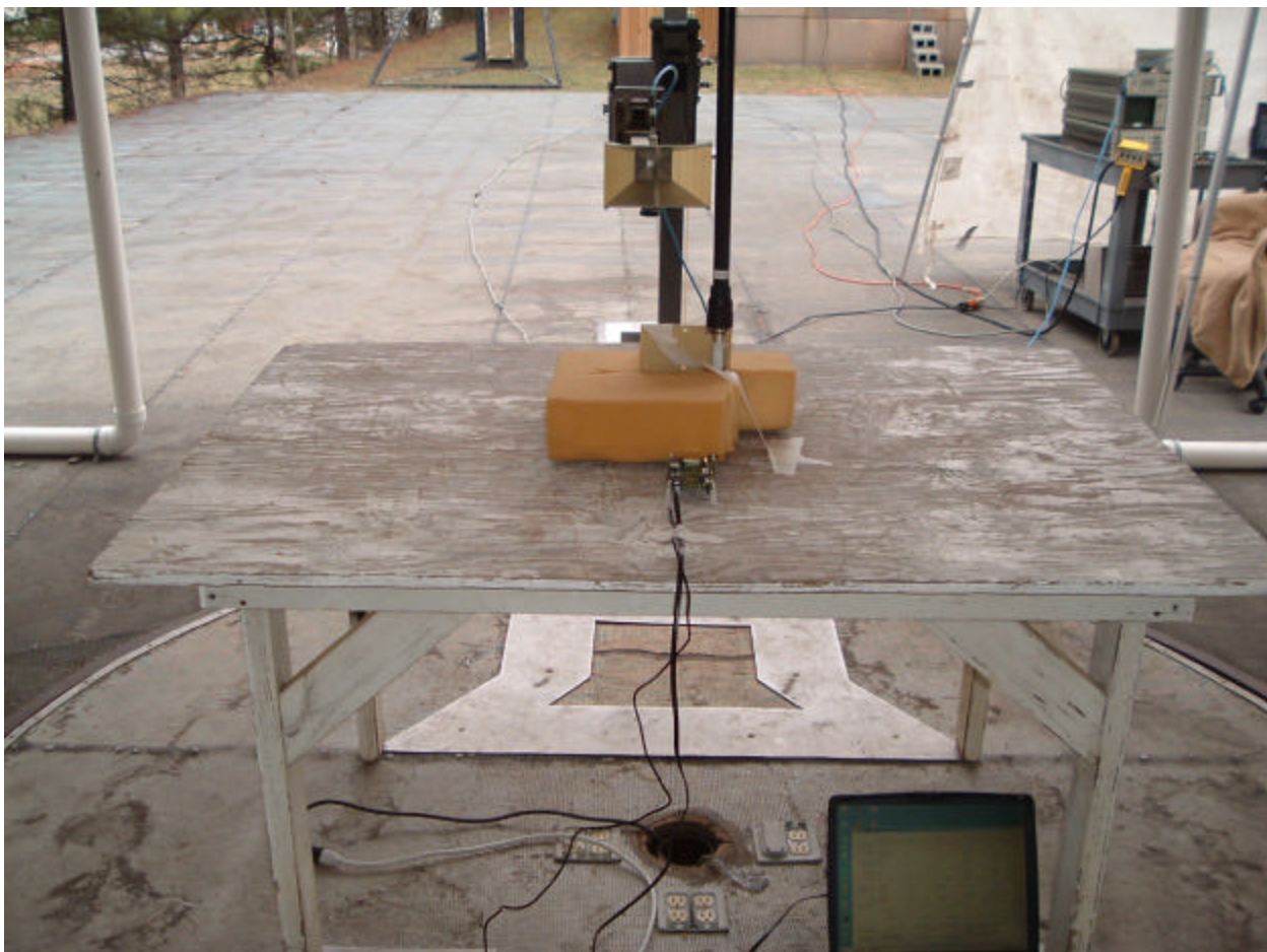
Photograph of Spurious Emissions Omni Antenna (Rear View)
