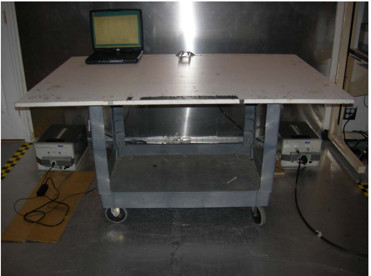
Figure 3: Test Setup – Conducted Emissions
