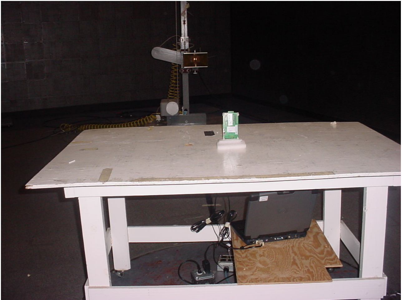
Figure 1: Test Setup – Radiated Emissions
