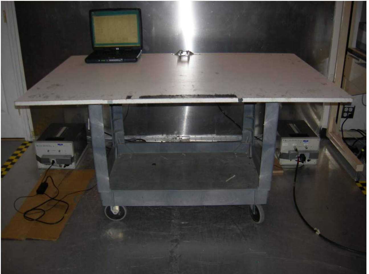
Figure 3: Test Set Up – Conducted Emissions
