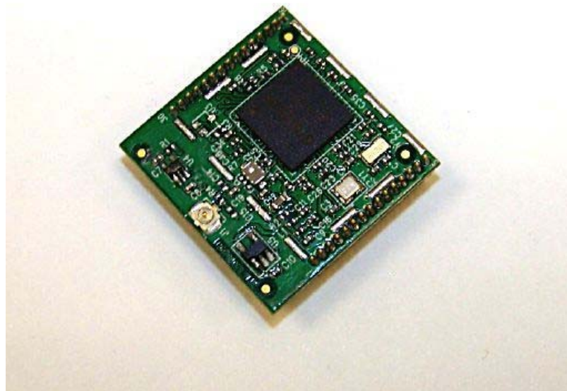
Original WSN802GP Module without Shield – Top View
