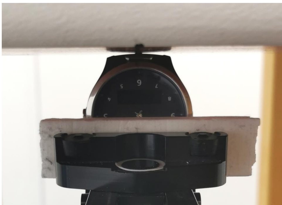
Bottom side of the device against the phantom, 0mm separation distance
