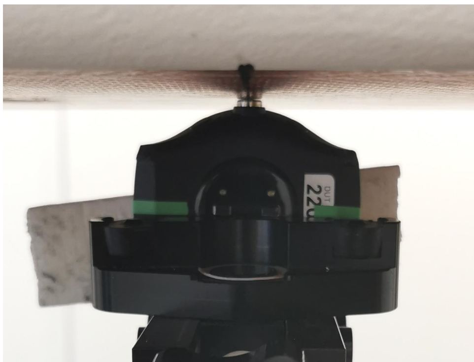
Right side of the device against the phantom, 0mm separation distance
