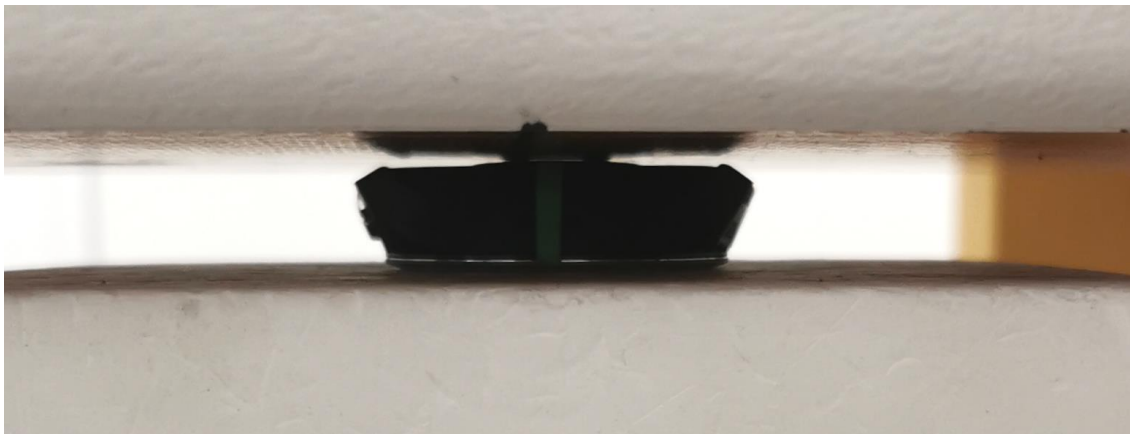
Back side of the device against the phantom, 0mm separation distance
