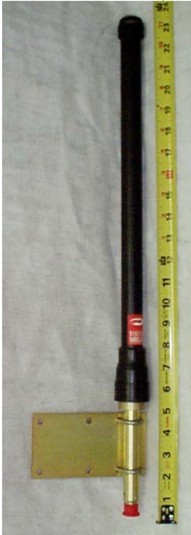
Photo 8. Antenna, Mobile Mark 6 dBi Omnidirectional (M/N OD6-2400-RTNC)
