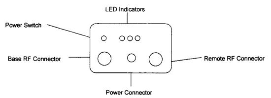
Proper placement of the external antenna is important since two modems inside the HN-2000 will be operating simultaneously. Be sure to physically separate the antennas from each other because the output transmission of one side of the repeater may interfere with the reception of the other. Use a remote cable between the repeater and each antenna, and space the antennas at least 2 meters apart.
