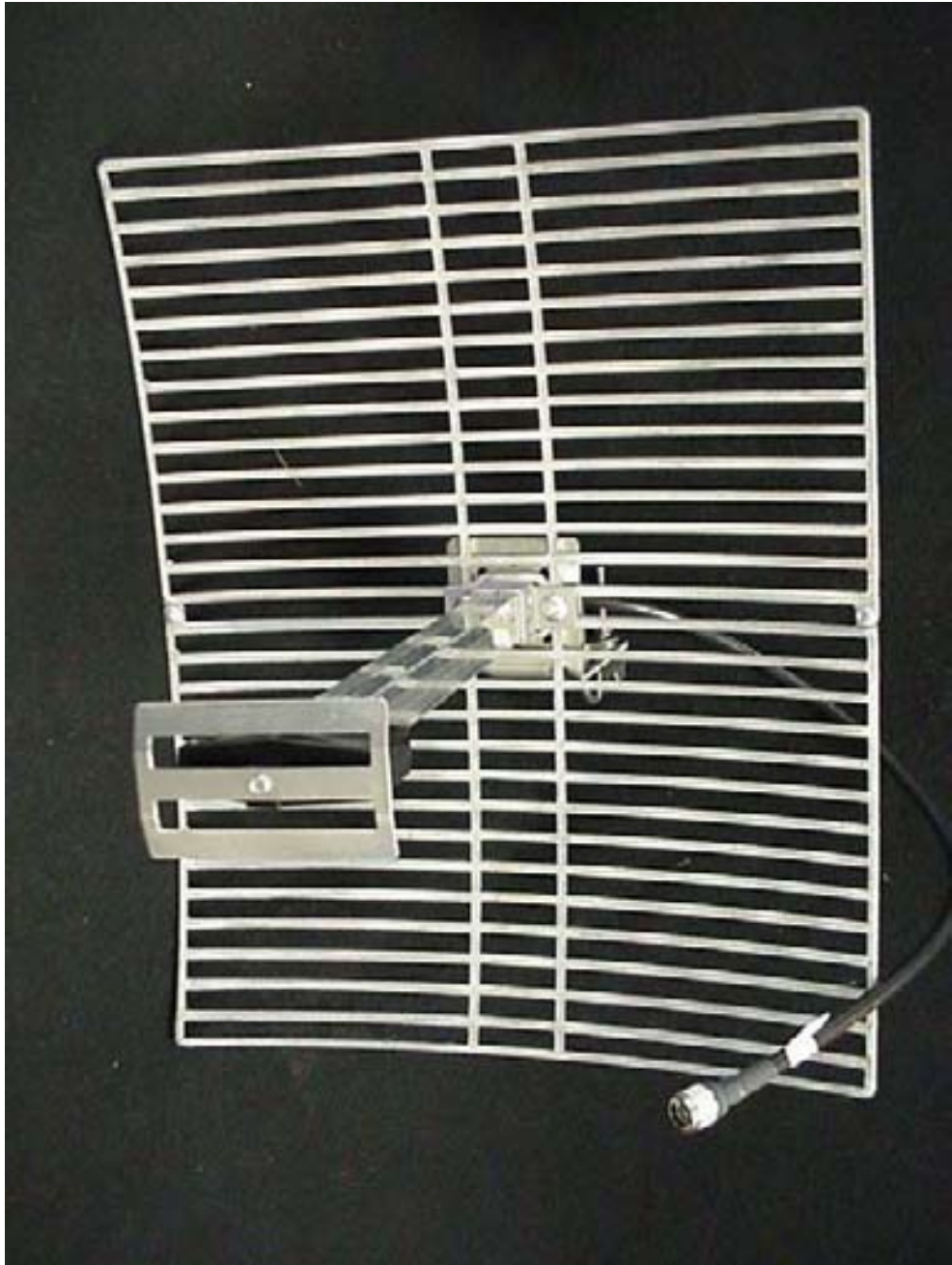
Photo 4. Antenna, Andrews 18 dBi Parabolic Dish (M/N 18T-2400 A)
