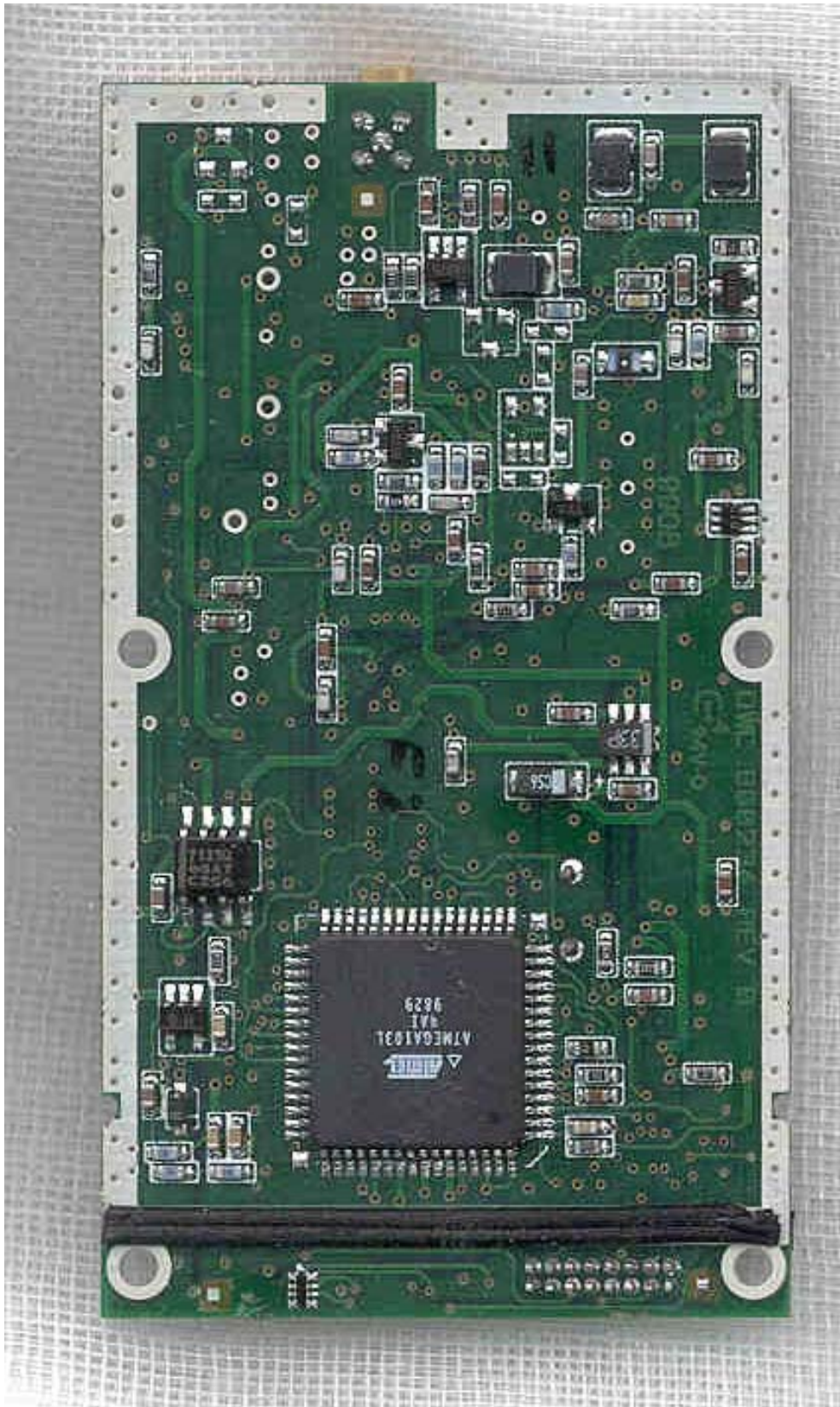
Photo 10. Modular Transceiver, Bottom View of Board
