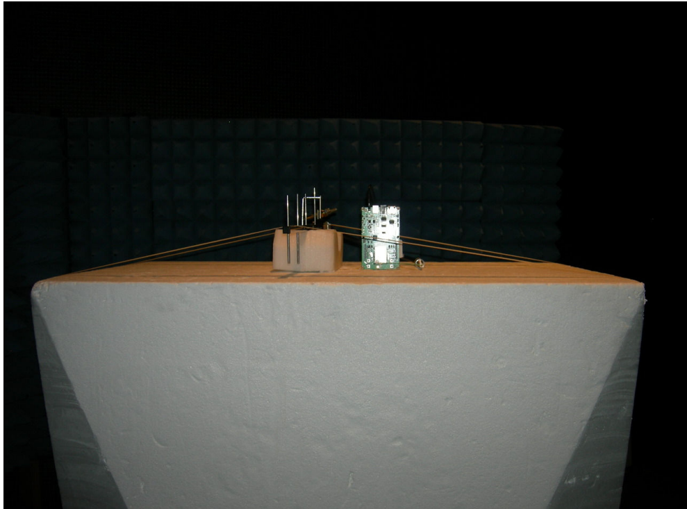
Figure 4: Radiated Emissions – Yagi Antenna
