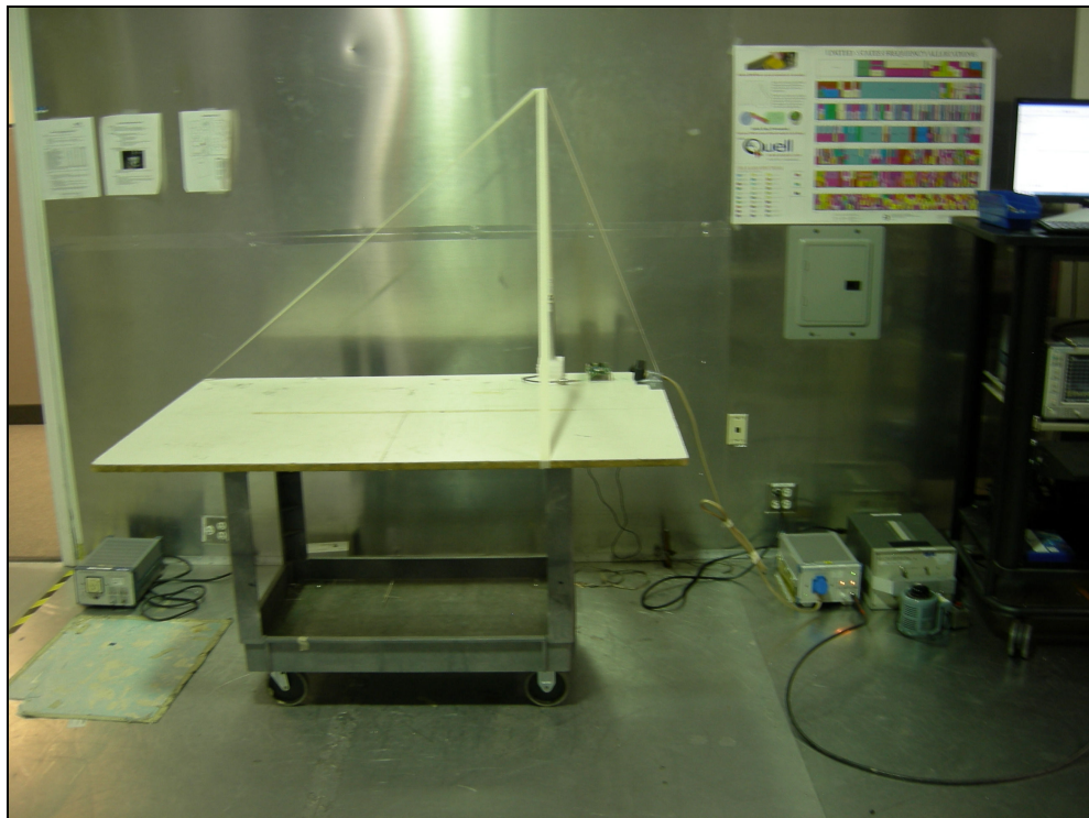
Figure 6: Conducted Emissions – Dipole Antenna
