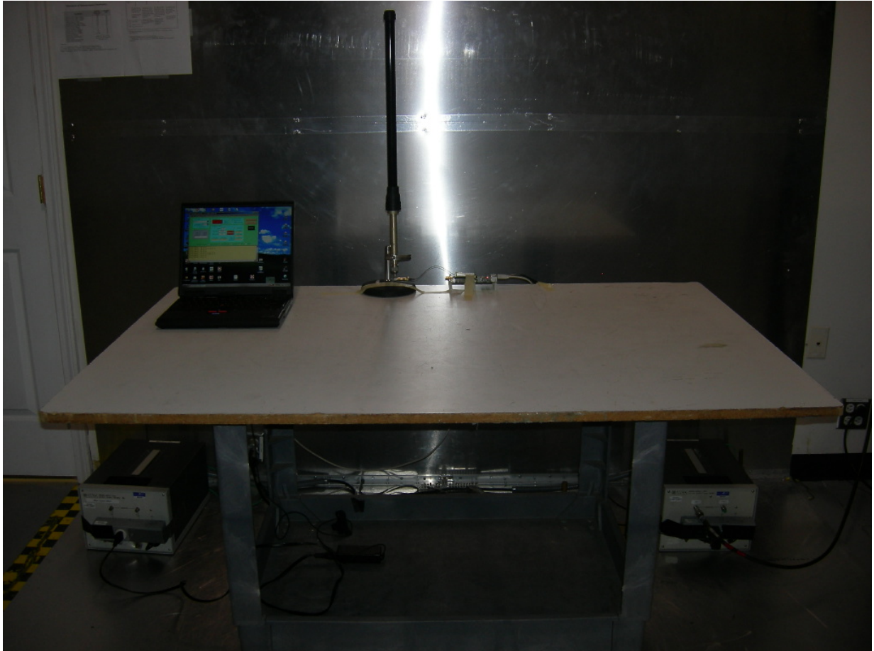
Figure 3: AC Power Line Conducted Emissions – Dipole Antenna
