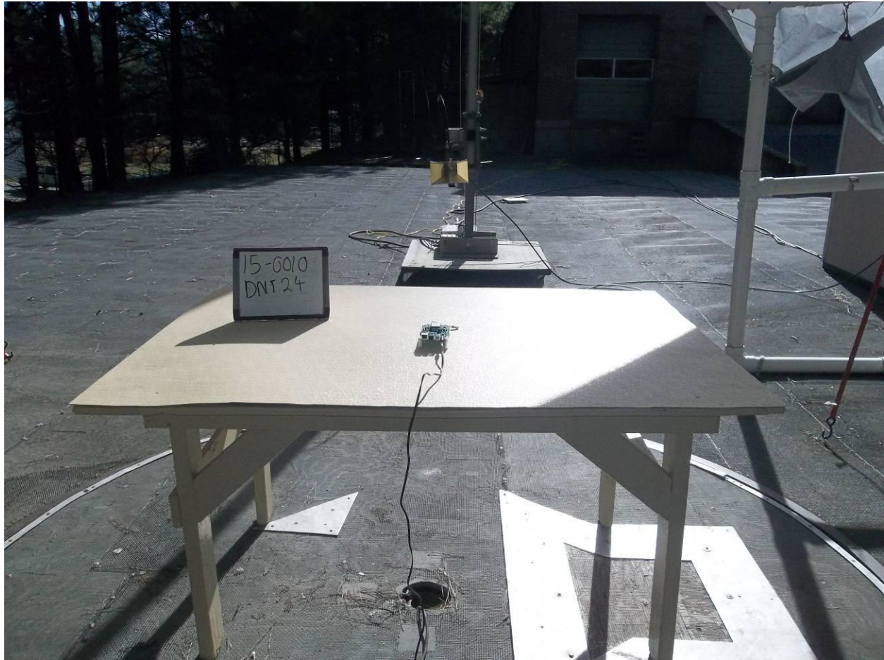
Figure 6. Radiated Emissions Test Setup, above 1 GHz, Back
