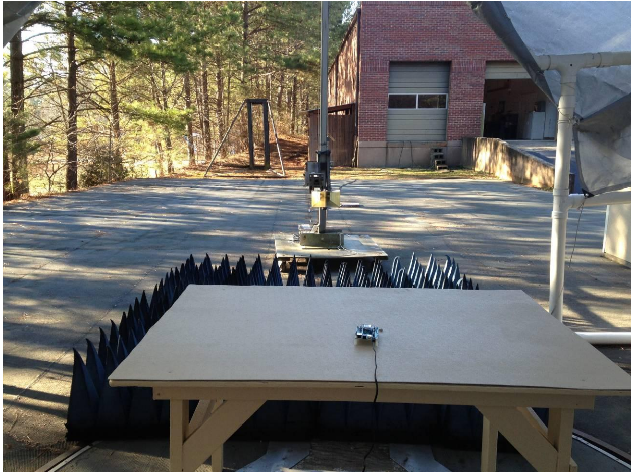
Figure 7. Radiated Emissions Test Setup, above 1 GHz, (per C63.4:2009 section 5.5)
