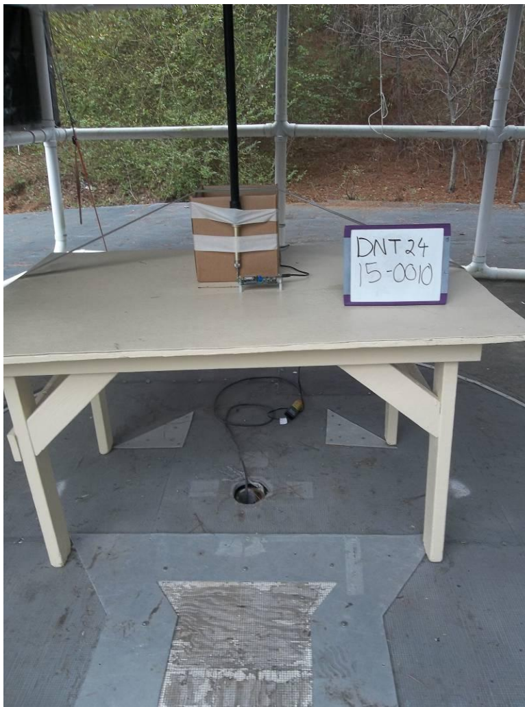
Figure 8. Radiated Emissions Test Setup, Spurious emissions with EUT connected to Omni Antenna, Front View (30 MHz to 1000 MHz)
