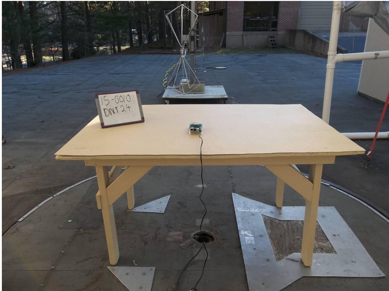
Figure 4. Radiated Emissions Test Setup, 30 MHz to 200Hz, Back
