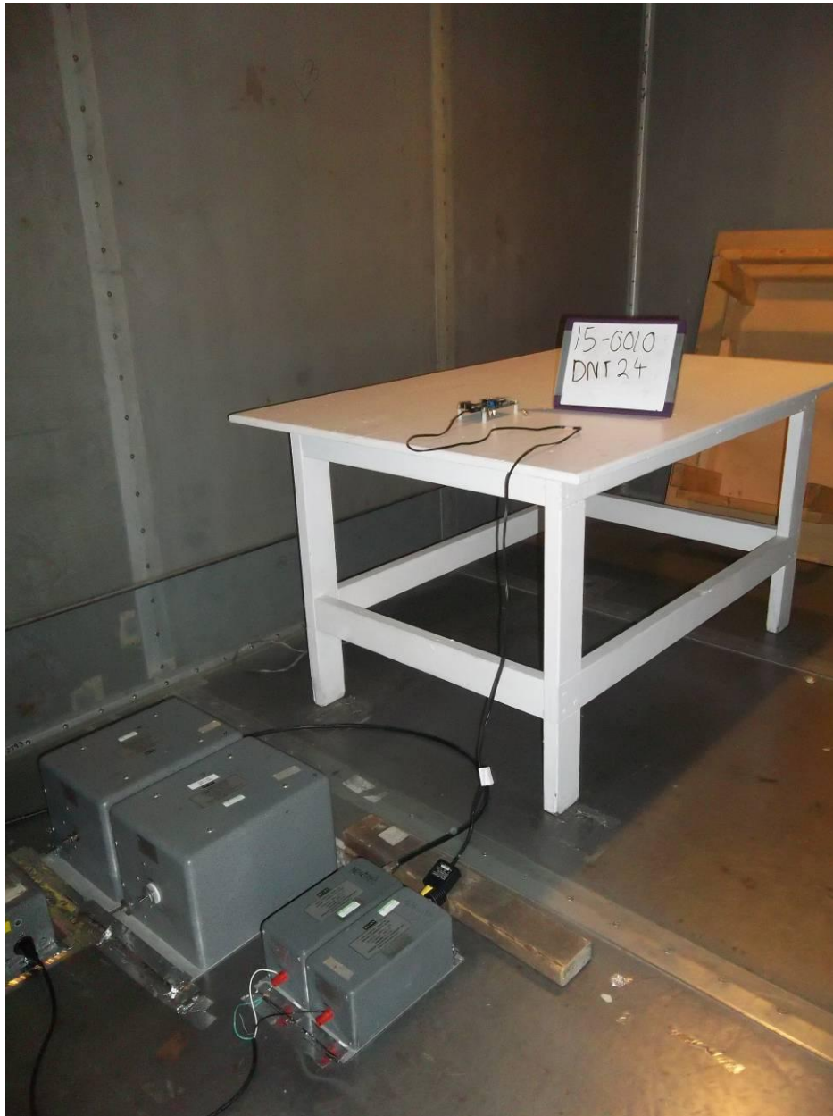
Figure 9. Conducted Emissions Test Setup
