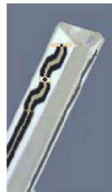
Figure 2.3 Probe Thick-Film Technique
