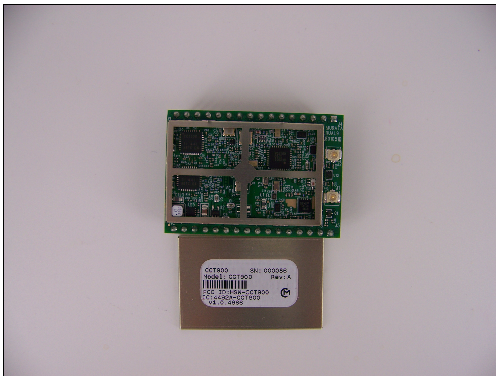
Figure 1: Internal Photo – Shields Removed
