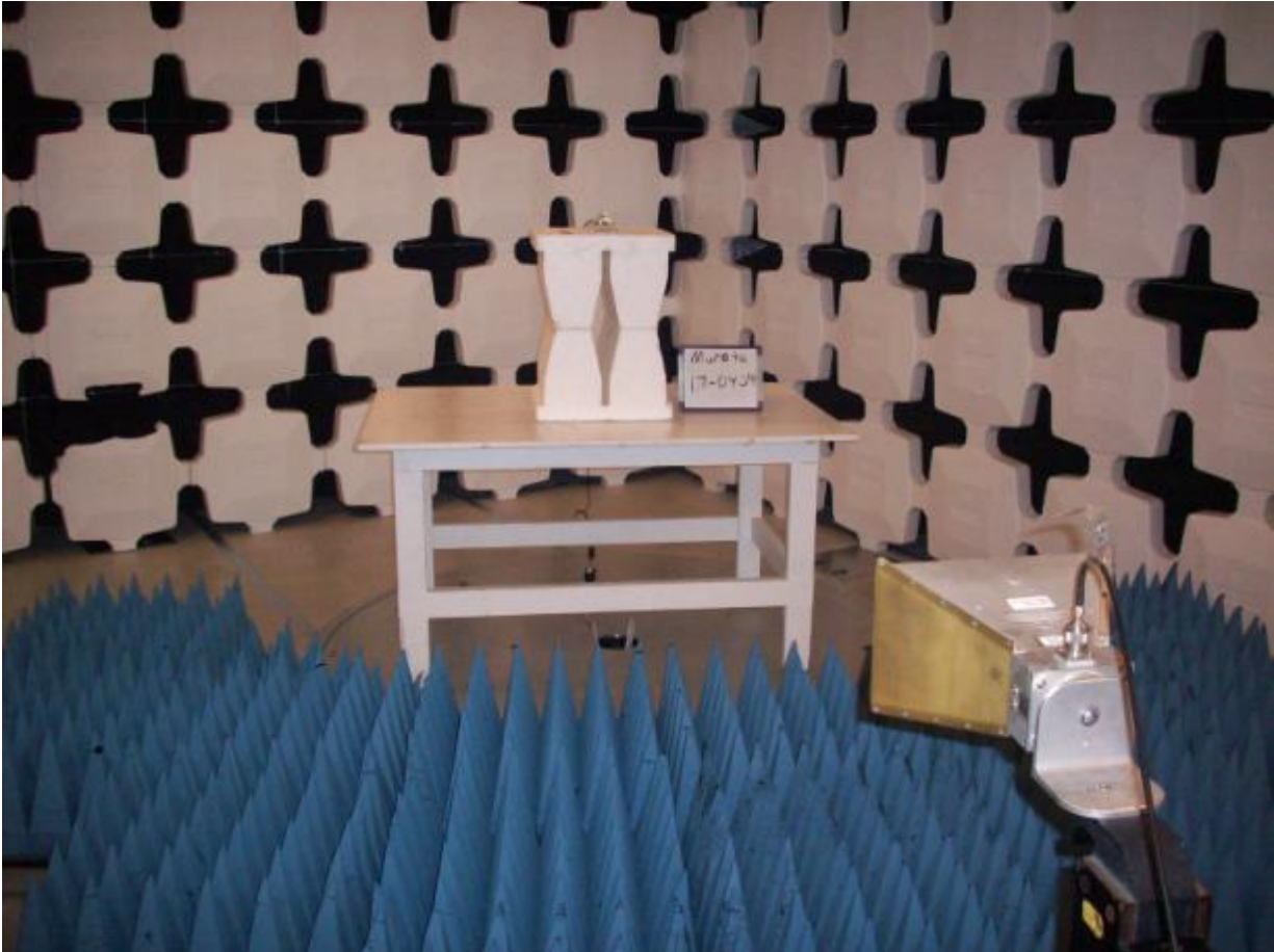
Figure 13. Spurious Emissions Configuration (> 1 GHz)
